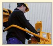
Levers for manual control of crawler in case of emergency
