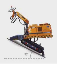
system assures that the correct spraying angle and a stable arm reach are maintained during the spraying process. The hydraulic blade-type stabilizer installed in the rear guarantees the equipment's stability in ascending slopes. In descending slopes, the electronically operated winch with 50 m cable and 6.803 kg traction force is applied.
