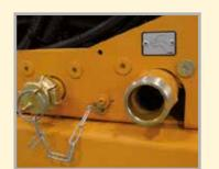
Quick couplings for concrete, additive and air supply. Without disturbing hoses on the sides of the machine
