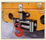
Tow coupling with a traction of 3.500 kg. Winch with 50 m cable and 6.308 kg capacity for secure work in steep descending slopes
